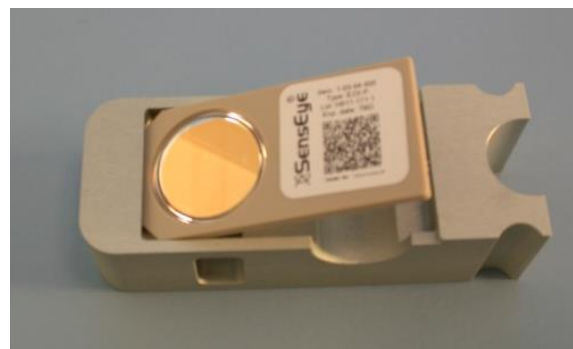
Figure 3. SensEye ® biosensor that will be inserted in the slider
